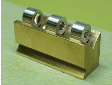
Figure 3.14: 3 lens subsystem. The lenses are placed in cylindrical mounts that have the exact same outer diameter to keep the lenses centered relative to each other. The v-groove allows only one translation.
