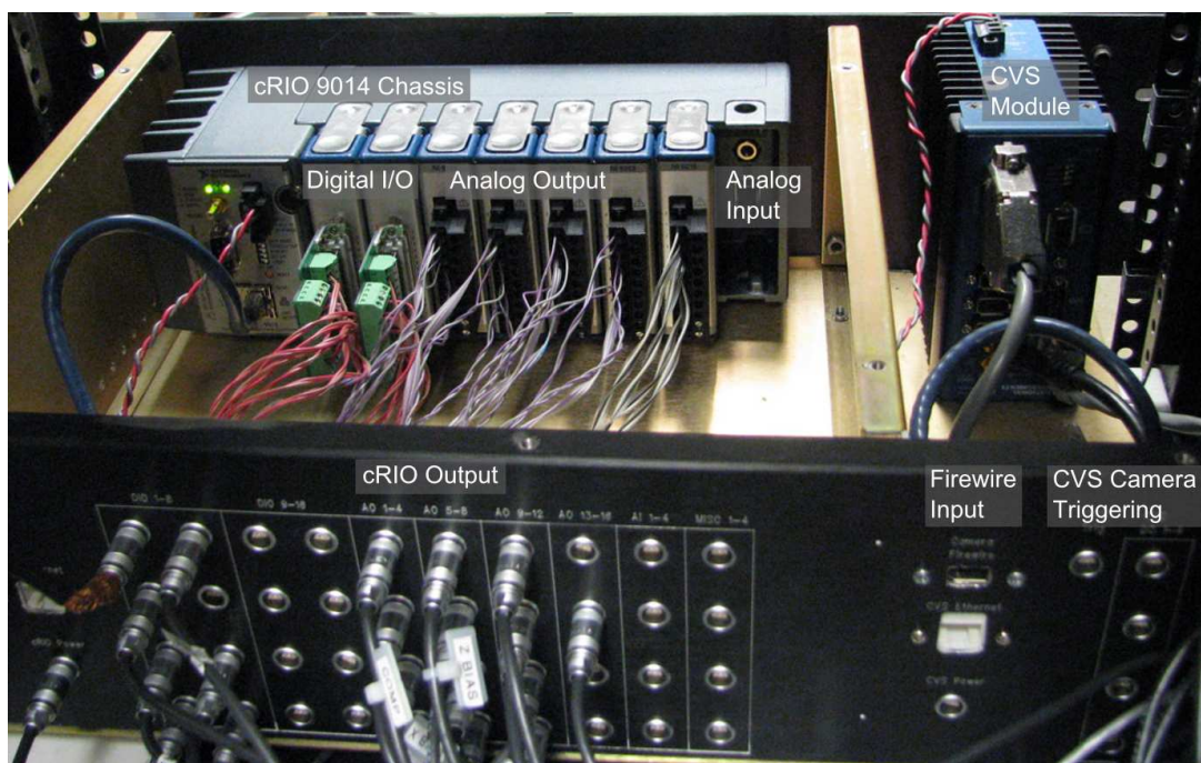
Figure 4.10: (Color) Photo of the cart computer control system. The left half of the box contains the NI cRIO. The right half of the box contains the NI CVS.
