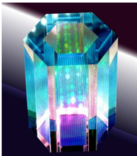
Figure 3.20: (Color) Photo of the AQuA cell hexagonal cell after polishing and AR coating.
